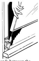
**NOTE:** Be careful not to place hands between the hinge and the oven door frame as the hinge could snap back and pinch fingers.
